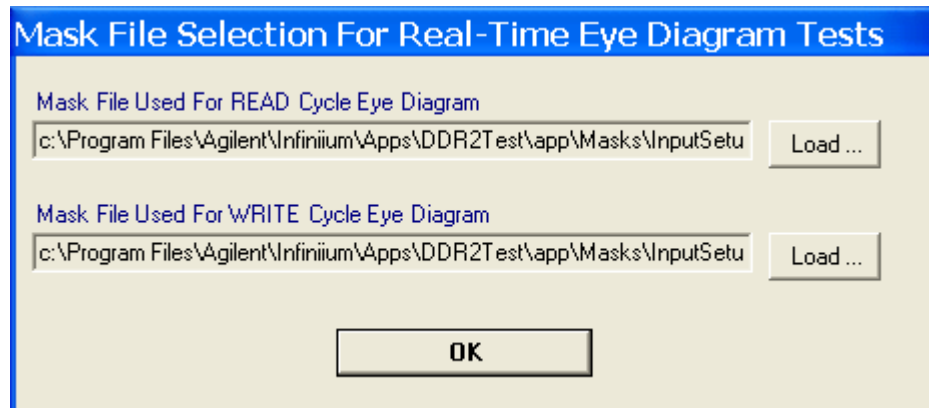
Figure 22 Selecting Test Mask for Eye Diagram Tests
